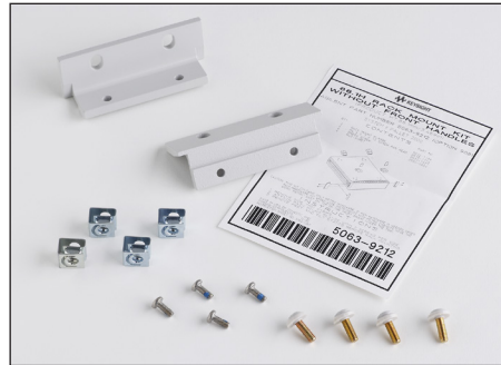
34191A 2U dual flange kit: secures the instrument to the front of the rack. This kit can be used with the 34194A dual lock link kit to mount two half-width, 2U height instruments side-by side.
